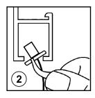
2. Tilt the track slide to insert into the underside of the track (can be fitted at any point along the track).
