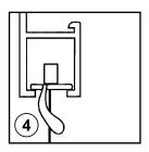
4. The hanger is now secure and ready for the adjustable hook to be fitted.
