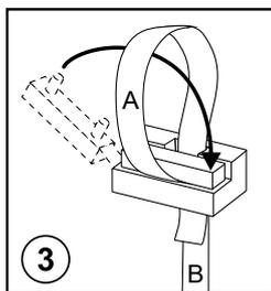
3. Pinch the capsule firmly with your fingers and then insert into the end of the track as shown with the locking bar to the front. (see Fig 2 & 3).
