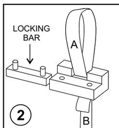
**IMPORTANT:** The short end must be to the front of the capsules as shown or the locking action will fail.
