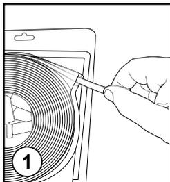
1. Pull tape from dispenser pack and cut off required length. Feed tape up through slot in the locking capsule and then back down through the same slot to form a large loop.
