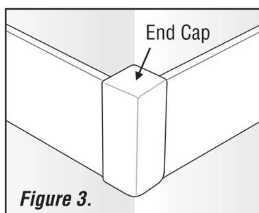
**NOTE:** INSIDE CORNERS do not expose the track ends, so End Caps are not required.
