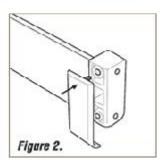
Push the End Cap into the end of the track as shown in Figure 1. Snap the twin covers in two and fit the single cover into the End Cap as shown in Figure 2. The curved part of the cover must face downwards.
