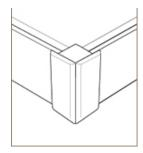
Push the End Cap into the end of the track as shown in figure 1. Fit the hinged cover as shown in Figure 3.
